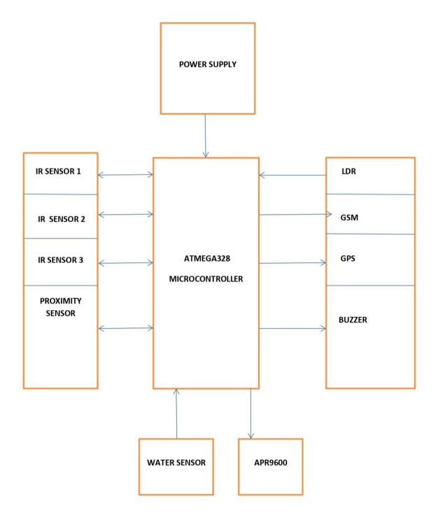
APR9600 is an IC used for sound recording .Recording is done in both serial and parallel ode.Sound output from microphone is fed to a pre amplifier and level of sound signal is measured. A non volatile RAM stores analog voltage. The diagram of a GSM system associated with the module is given below.
